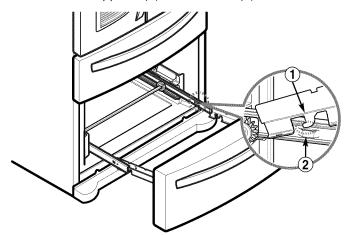
3. Lower door into final position and tighten the screws(3). Make sure you have a right rail cover for each side.
